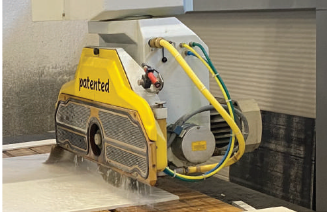
Figure D-1: Use Water to Cool Blade and Slab
