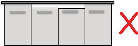
Figure C-1: Improper Support (No direct support)
