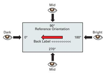
Figure D-1 - Effect of Orientation on Reflectivity
